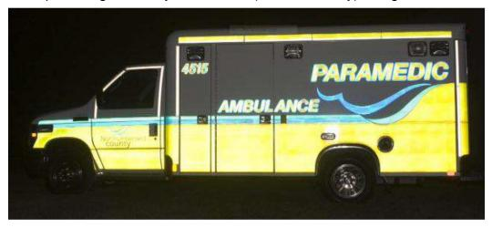
The difference above is quite noticeable. On the high visibility ambulance, a reflective white stripe outlines the cab and body showing the size and shape of the vehicle. The high visibility green at the top of the box outlines the vehicle and adds to side visibility, especially during traffic movement. Large block lettering allows the vehicle to be easily identified. As per requirement of the Ambulance Act, the lettering is also highly contrasted.
